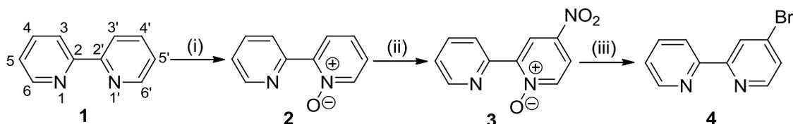
**Scheme 1:** Preparation of 5-alkynylbipyridine ligands. *Conditions:* (i) *m*-CPBA, CHCl<sub>3</sub>, 40 °C, 24 h; (ii) HNO<sub>3</sub> 100%, H<sub>2</sub>SO<sub>4</sub>, reflux, 6 h; (iii) CH<sub>3</sub>COBr/CH<sub>3</sub>COOH, rt, 30 min., then PBr<sub>3</sub>, 40 °C then 100 °C for 1 h
