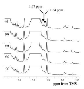
Fig. 3: Expanded <sup>1</sup>H-NMR spectra for sol fraction of commercial NR (a) PC-TE, (b) RSS3-TE,
