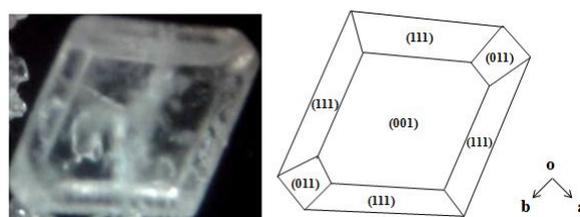
Figure 4: Schematic surfaces of  $\alpha$ -form crystal
