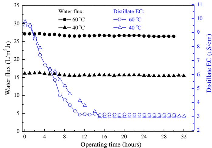
Figure 6: Water flux and distillate electrical conductivity (EC) during DCMD of seawater at a constant water recovery of 70 % with scaling mitigation techniques
