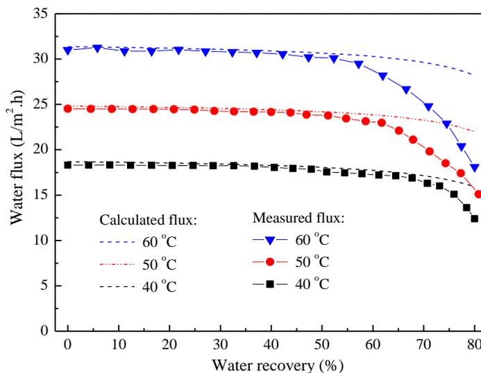
Figure 4: Calculated and experimentally measured water flux as functions of water recovery during DCMD of pre-filtered seawater. Operating conditions: distillate temperature,  $T_{distillate}$ , of 25 °C, water circulation rates  $F_{feed} = F_{distillate} = 1.0$  L/min
