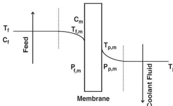
Figure 2: Temperature and concentration polarization effects in DCMD (adapted from [4])
