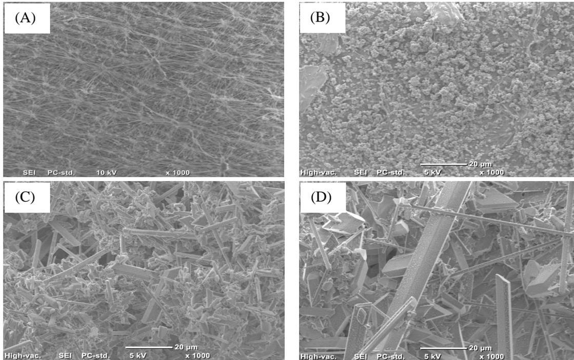
Figure 5: SEM images of (A) a virgin membrane and scaled membrane at the end of the DCMD process with pre-filtered seawater at feed temperature of (B) 40 °C, (C) 50 °C, and (D) 60 °C
