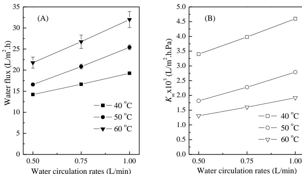
Figure 3: The influence of feed temperature and water circulation rates on (A) water flux and (B) the mass transfer coefficient of the DCMD system with Milli-Q water at a constant distillate temperature,  $T_{distillate}$ , of 25 °C
