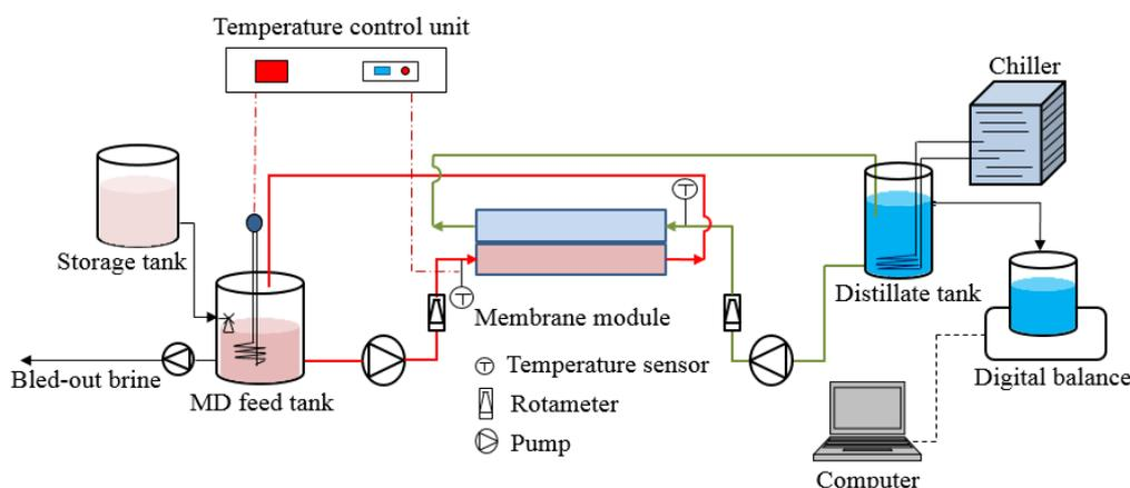
Figure 1: The schematic diagram of the lab-scale DCMD system
