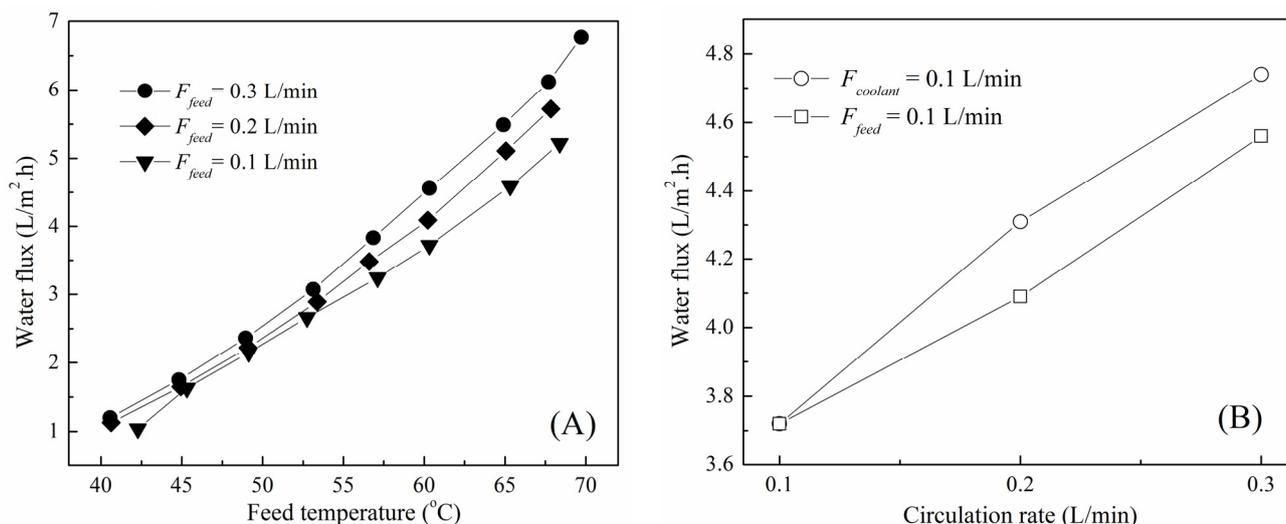
Figure 1: The influences of feed temperature and circulation rates on water flux of the AGMD process with the synthetic NaCl solution at: (A) coolant temperature  $T_{coolant} = 25$  °C, coolant circulation rate  $F_{coolant} = 0.1$  L/min, and (B) feed temperature  $T_{feed} = 60$  °C, coolant temperature  $T_{coolant} = 25$  °C
