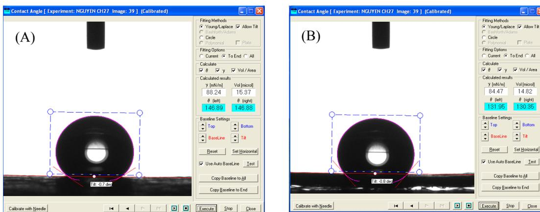
Figure 4: Contact angles of (A) the virgin membrane and (B) the fouled membrane after cleaning with vinegar
