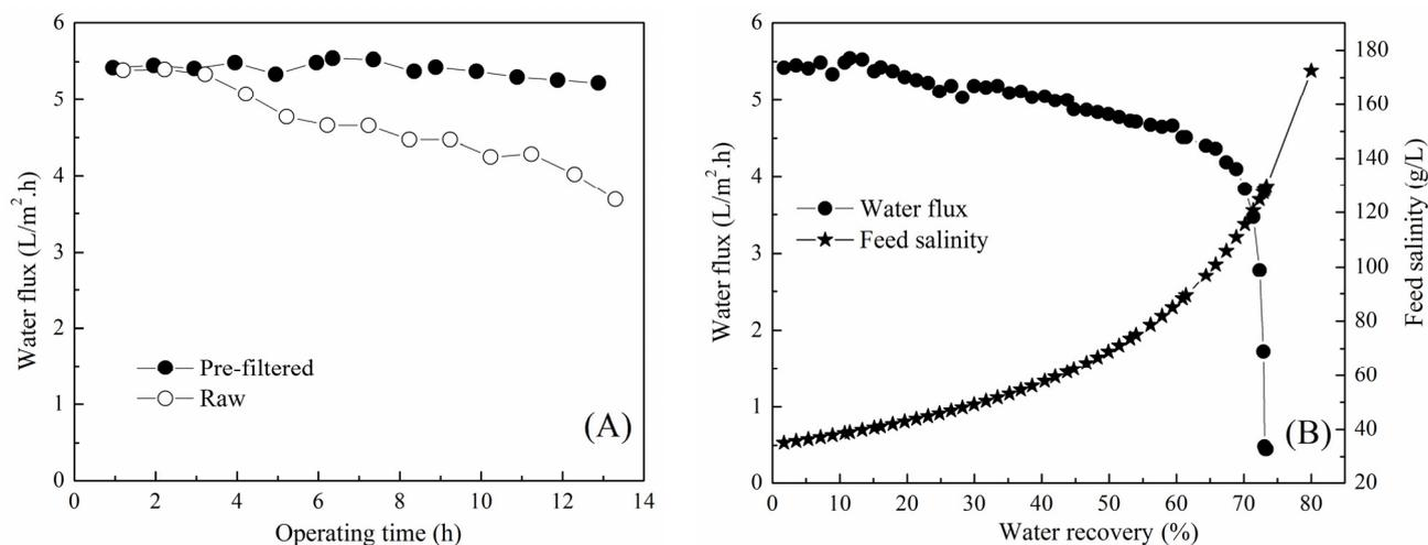
Figure 2: (A) Water flux of the AGMD process with raw and pre-filtered seawater feed, and (B) water flux and feed salinity versus water recovery during the durable AGMD process of pre-filtered seawater feed. Operating conditions: feed temperature  $T_{feed} = 60\text{ }^{\circ}\text{C}$ , distillate temperature  $T_{distillate} = 25\text{ }^{\circ}\text{C}$ , water circulation rates  $F_{feed} = F_{distillate} = 1.0\text{ L/min}$
