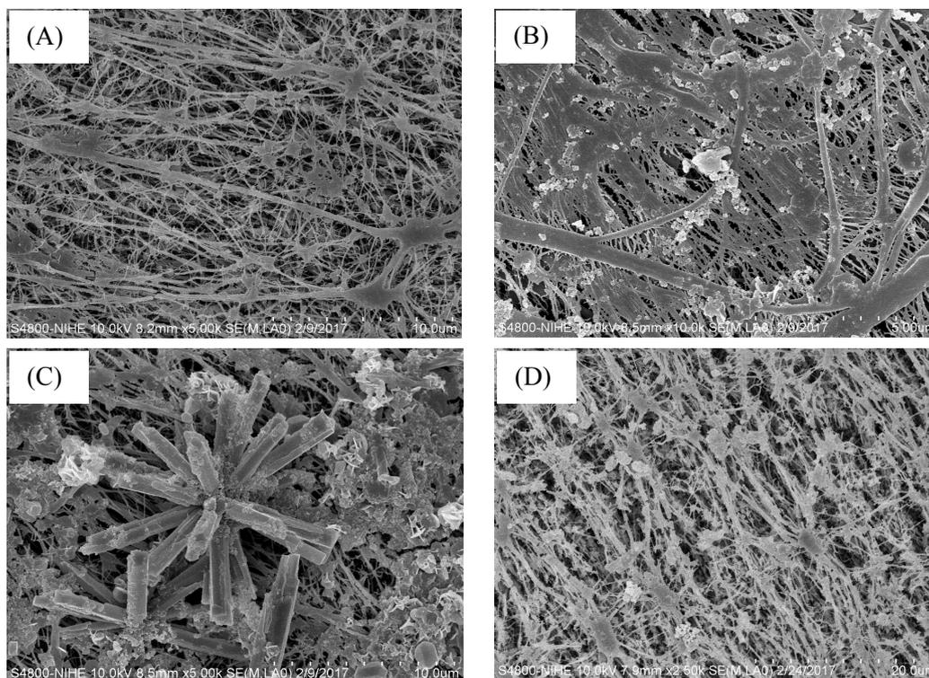
Figure 3: SEM images of: (A) a virgin membrane, (B) membrane fouled with organic matters, (C) membrane scaled with sparingly soluble salts, and (D) the scaled membrane after cleaning with vinegar
